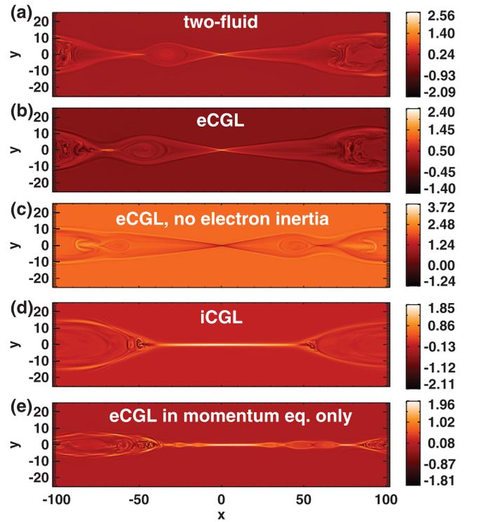
FIG. 1. Out-of-plane current density  $J_z$  using various models: (a) two-fluid, (b) eCGL, (c) eCGL with no electron inertia, (d) iCGL, (e) eCGL in the momentum equation only.
