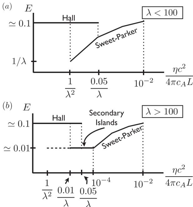
FIG. 3. Expected bifurcation diagram of 2D reconnection for (a)  $\lambda < 100$  (sketched for  $\lambda \simeq 50$ ) adapted from Refs. 54 and 70 and (b)  $\lambda > 100$  (sketched for  $\lambda \simeq 1,000$ ).
