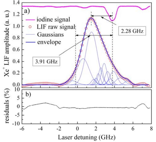
FIG. 7. Parallel LIF measurement of  $\text{Xe}^+$ : the red symbols are the raw LIF signal, the blue thin lines are Gaussian fits to the 15 components, the blue thick line is the envelope of the fits, and the magenta line is the iodine reference spectrum.
