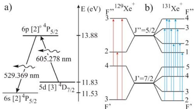
FIG. 1. a) Three-level Xe<sup>+</sup> LIF scheme; b) hyperfine structure of 605.278 nm line of the odd isotopes due to nuclear spin splitting.
