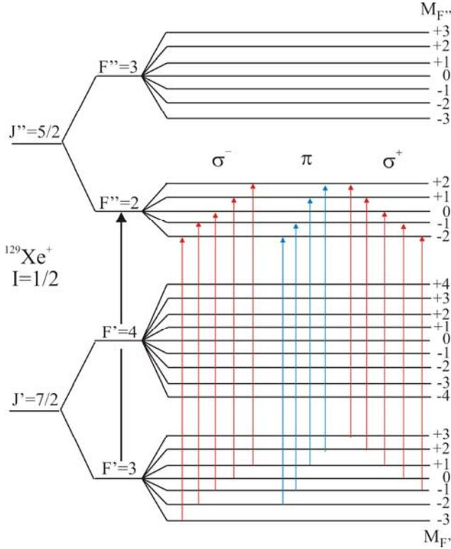
FIG. 4.  $^{129}\text{Xe}^+$   $5d\ ^4D_{7/2}(F'=3) \rightarrow 6p\ ^4P_{5/2}(F''=2)$  Zeeman line splitting.
