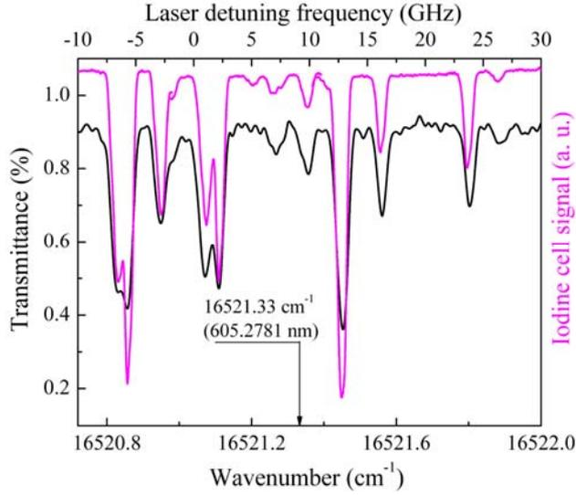
FIG. 6. The experimental iodine spectrum (magenta) and the absorption iodine spectrum (black) according to Ref. [9]. The arrow indicates the absolute wave number of the 605.2781 nm  $\text{Xe}^+$  line.
