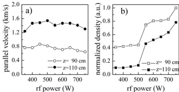
FIG. 8. a) Xe<sup>+</sup> parallel flow speed and b) the normalized Xe<sup>+</sup> density estimated from the LIF signal amplitude.
