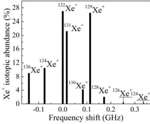
FIG. 2.  $\text{Xe}^+$  isotopic abundance and frequency shifts relative to  $^{132}\text{Xe}^+$  for the  $5d\ ^4\text{D}_{7/2} \rightarrow 6p\ ^4\text{P}_{5/2}$  transition [5].
