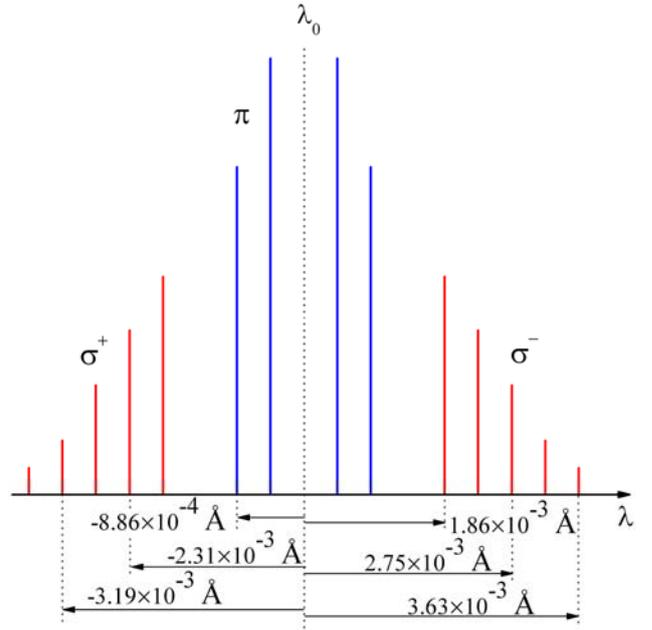
FIG. 5.  $^{129}\text{Xe}^+$  Zeeman shifts for  $F'=3 \rightarrow F''=2$  hyperfine transition of the  $\lambda_0=605.278$  nm line.
