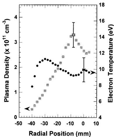
FIG. 3. Plasma density (circle) and electron temperature (square) as a function of the radial position in the plasma column. Discharge conditions:  $|B| = 1$  KG, Pressure=6.5 mTorr, Power=400 Watts.
