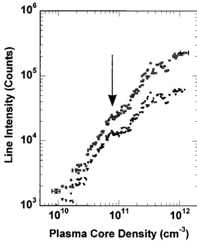
FIG. 5. Triplet (square) and singlet (triangle) integrated line intensities as a function of plasma density. The slope of the two signals remains the same up to a density of  $8 \times 10^{10} \text{ cm}^{-3}$  (arrow), then the two slopes diverge.
