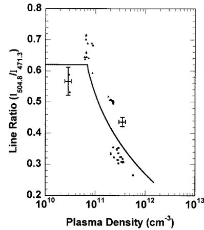
FIG. 7. Line ratio as a function of plasma density. Fit (solid line) for the  $10 \text{ eV}$  line ratio function as obtained from the experimental data (see Sec. IV).  $7 \text{ eV}$  line ratio values (solid circle),  $12 \text{ eV}$  line ratio values (solid triangle).
