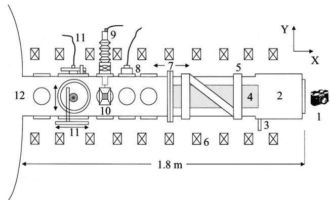
FIG. 1. Upper view of the HELIX plasma source. 1. Digital camera (near axial viewport), 2. Pumping station, 3. Gas inlet, 4. Plasma column, 5. Fractional helix antenna, 6. Magnetic field coils, 7. Glass chamber section (right), SS chamber section (left), 8. Spectroscopy optics, 9. Retractable rf compensated Langmuir probe, 10. Microwave interferometer, 11. 2D LIF injection and collection optics, 12. Large space chamber.
