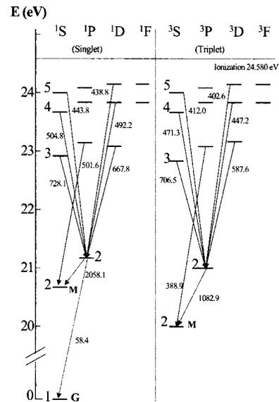
FIG. 2. Partial Grotrian diagram of the helium atom with some important transitions ( $\lambda$  in nm). Visible transitions (full line), infra red, and ultraviolet lines (hash line). G and M are for ground and metastables states, respectively.
