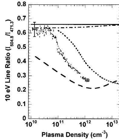
FIG. 6. 10 eV Line ratio (504.8/471.3) as a function of plasma density. Experimental line ratios (solid circle), SSC model (solid line), SSC model + metastable contributions (alternative dot-dash line), corrected Sasaki CR model (large dash line), and Brosda CR model (dotted line).
