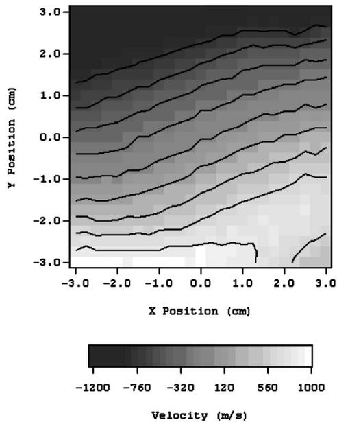
FIG. 3. Contours of constant  $V_{ix}(x,y)$  in the center of the discharge for a source magnetic field of 652 G, rf power of 750 W, and a neutral pressure of 1.7 mTorr.
