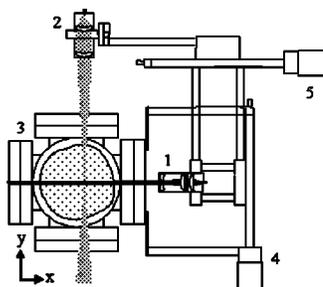
FIG. 2. The 2D scanning apparatus: (1) Beam reducing and polarizing injection optics, (2) optimized collection optics, (3) plasma source chamber, (4) Y-axis scanning stage, and (5) X-axis scanning stage.
