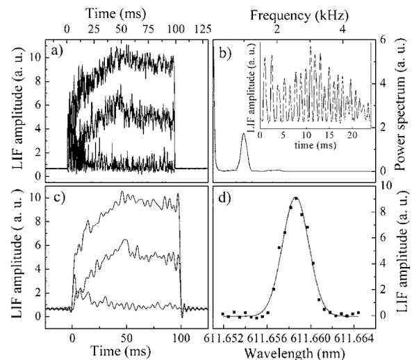
FIG. 3. (a) Raw LIF signal during the 100 ms discharge pulse (only 3 of 25 wavelengths are plotted). (b) Oscillations of the LIF signal amplitude observed on the first 26 ms of the pulse (as insert) and corresponding power spectrum showing 1 kHz oscillation frequency. (c) LIF signal after low pass filtering. (d) Argon ion vdf at  $t=50 \text{ ms}$  into the pulse.
