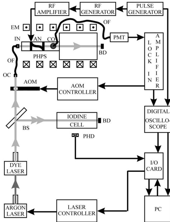
FIG. 1. Experimental setup for time resolved LIF diagnostic: PHPS—pulsed helicon plasma source, IN—injection optics, AN—antenna, CO—collection optics, BD—beam dump, EM—electromagnets, PMT—photomultiplier tube, OF—optical fiber, OC—optical coupler, AOM—acousto-optic modulator, PHD—photodiode, and BS—beam splitter.
