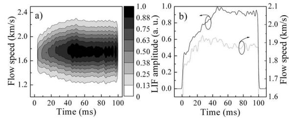
FIG. 4. (a) Contour plot of the evolution of the argon ion vdf during the 100 ms pulse with 100  $\mu\text{s}$  time resolution. (b) Evolution of the LIF signal amplitude (continuous line) and ion flow velocity (dashed line) during the pulse.
