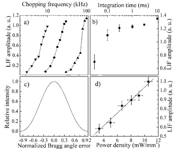
FIG. 2. (a) The LIF signal amplitude dependence vs chopping frequency ( $2\text{--}100 \mu\text{s}$ ,  $300 \mu\text{s}$ ,  $1\text{--}1 \text{ ms}$  integration times). (b) The LIF signal amplitude dependence vs integration time for 100 kHz chopping frequency. (c) The relative intensity of the AOM transmitted light in the first diffraction order vs Bragg angle misalignment. (d) The dependence of LIF signal amplitude vs injected laser power density.
