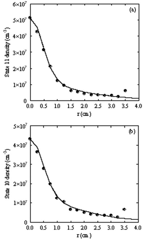
**Figure 8.** Neutral argon excited state density versus radial position, comparison between experimental data (circles) and CR model output (solid lines) for (a) State 11 and (b) State 10.
