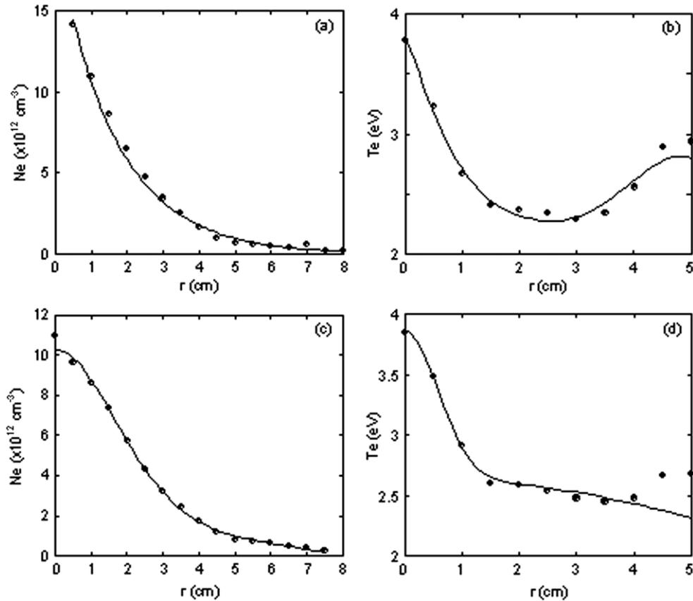
**Figure 5.** Langmuir probe data with the fits used for CR model inputs for case A (300 W rf power, 750 G magnetic field, 6.0 mTorr fill pressure/18.7 mTorr operating pressure): (a) electron density and (b) electron temperature. For case B (350 W rf power, 750 G magnetic field, 5.1 mTorr fill pressure/15.1 mTorr operating pressure): (c) electron density and (d) electron temperature.
