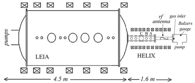
**Figure 1.** Schematic of HELIX indicating location of (A) Baratron gauge, (B) Langmuir probe and (C) LIF and spectroscopy collection optics.
