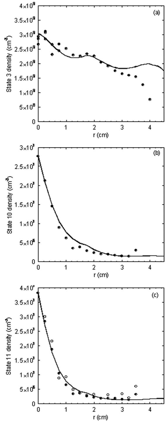
**Figure 4.** Neutral argon excited state density versus radial position, comparison between experimental data (circles) and CR model output (solid line) for a 3 cm wide depletion of 60%. (a) State 3. (b) State 10. (c) State 11. In (c) the nearly identical measured profiles for the 668 nm (open circles) and 751 nm (filled circles) transitions are shown.
