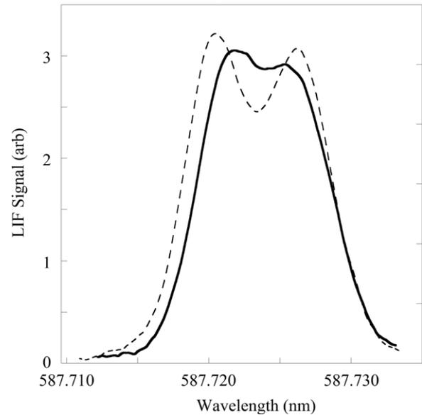
**Figure 10.** On-axis, parallel neutral helium LIF measurement for a static (solid line) and flowing (dashed line) discharge. The same laser power was used for both measurements at  $z = 100 \text{ cm}$ .
