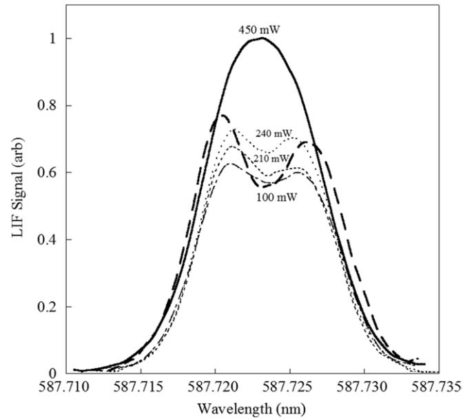
**Figure 6.** On-axis, parallel neutral helium LIF measurements as a function of injected laser power, 100 cm downstream of the rf antenna. The laser powers, starting from the topmost curve, are 450, 240, 210, 170 (unlabeled) and 100 mW.
