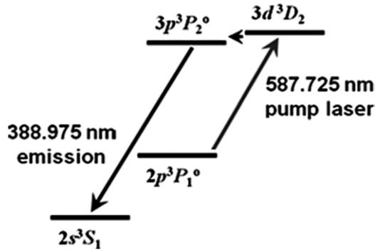
**Figure 3.** The four-level neutral helium LIF scheme used in these experiments. After being excited to the  $3d^3D_2$  state, electrons are knocked into the  $3p^3P_2$  state through collisional processes. Wavelengths shown are the vacuum values.
