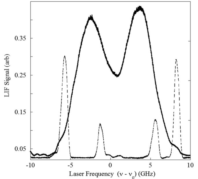
**Figure 4.** Typical on-axis, parallel neutral helium LIF measurement (solid line) obtained 85 cm downstream of the driving antenna. The simultaneously measured fluorescence spectrum of molecular iodine (dashed line) provides an absolute flow velocity reference.
