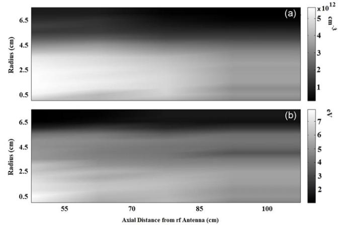
**Figure 2.** Smoothed plots of the measured (a) electron density and (b) electron temperature versus radial location and distance from rf antenna.
