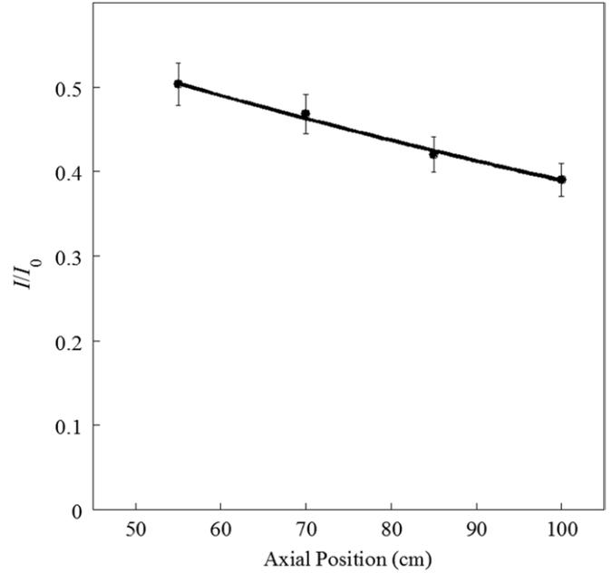
**Figure 8.** The ratio of the dip at the center of the on-axis VDF measurements,  $I/I_0$ , extracted from each normalized VDF plotted versus the four axial distances. Also shown is an exponential fit to the measurements.
