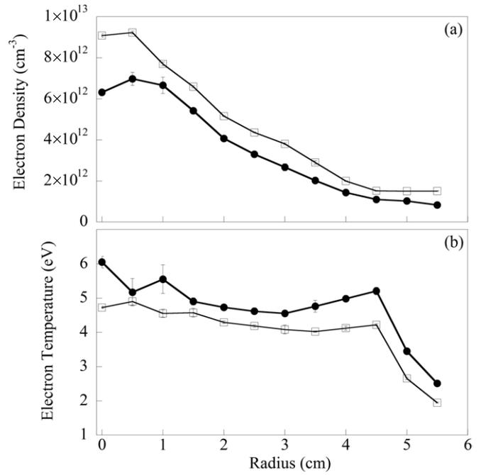
**Figure 9.** (a) Electron density versus radius for the flowing gas with active pumping (filled circles) and static (open squares) discharges at 18 mTorr. (b) Electron temperature versus radial location for the same two cases.
