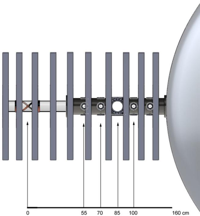
**Figure 1.** Schematic of the HELIX-LEIA apparatus (a portion of the end of the LEIA chamber is shown at the right of this figure). The 19 cm long  $m = 1$  antenna surrounds the glass portion of the chamber at  $z = 0$  cm. Ten electromagnets, aligned as shown, provide the magnetic field in the source region. The parallel laser injection optic was placed at  $z = -100$  cm. Fluorescent emission was collected at distances of 55, 70, 85 and 100 cm downstream of the rf antenna.
