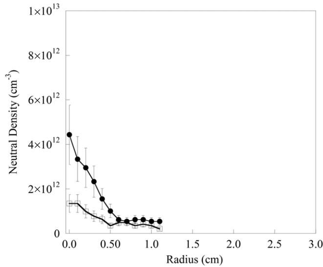
**Figure 11.** Neutral density versus radial location for two different fueling configurations, flowing gas with active pumping (filled circles) and ‘static,’ no pumping (open squares).
