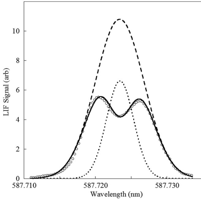
**Figure 7.** A typical on-axis, LIF measurement of the VDF (open circles) and a nonlinear fit (solid line) of assuming a Maxwellian 'parent' VDF (dashed line) and a Gaussian absorption feature (dotted line). The ratio of the dip's depth ( $I$ ) to the amplitude of the parent LIF VDF ( $I_0$ ) is used to determine the neutral density; as explained in the text.
