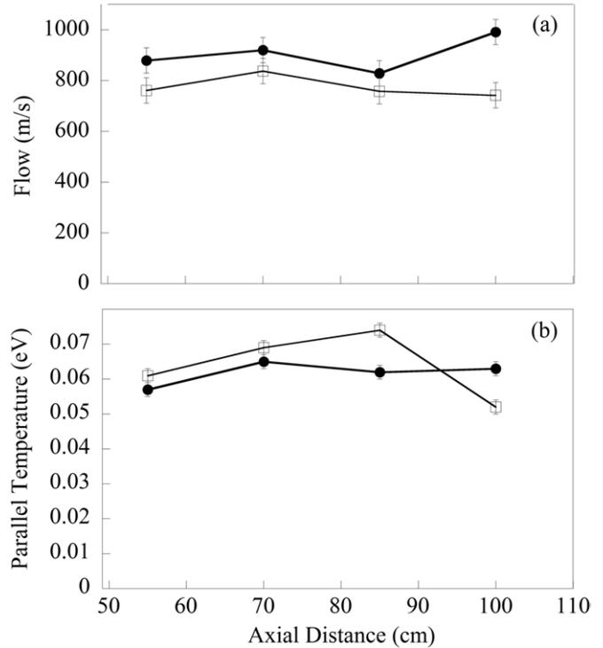
**Figure 12.** (a) Parallel, on-axis neutral velocity versus distance along the axis of the source for the flowing gas (filled circles) and static (open squares) fueling configurations. (b) The parallel neutral temperatures for the same fueling cases.
