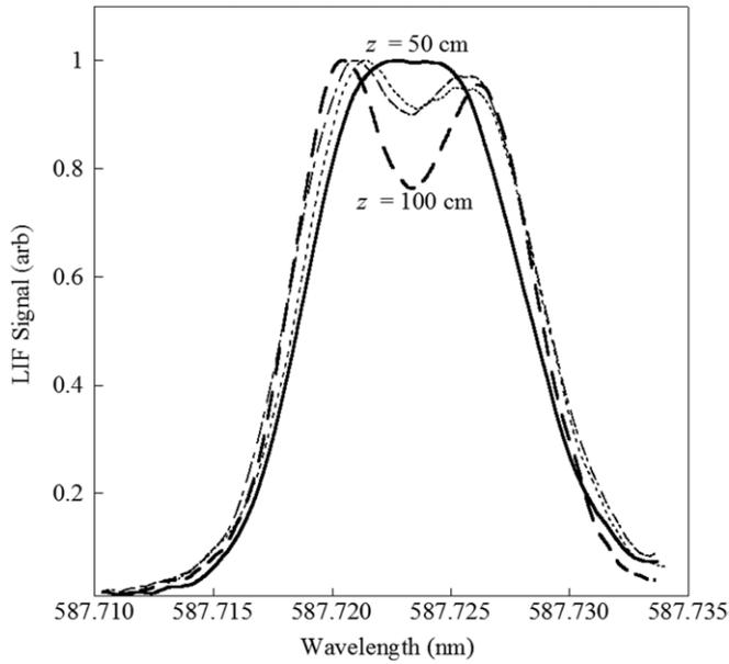
**Figure 5.** On-axis VDF measurements at axial locations of 55 (solid line), 70, 85 and 100 cm (dashed line) downstream of the driving antenna. The ‘dip’ in the VDF increases with increasing distance.
