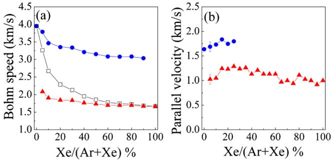
FIG. 3. (Color online) (a) Individual ion sound speeds (circles for Ar<sup>+</sup> and triangles for Xe<sup>+</sup>) and the system sound speed (open squares) as function of xenon fraction in HELIX at  $z=126$  cm. (b) Parallel ion flow speeds in HELIX at  $z=126$  cm vs xenon fraction (same symbol assignment).
