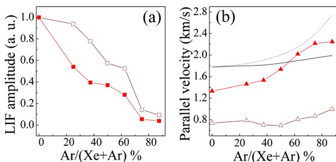
FIG. 6. (Color online) (a) Normalized  $\text{Xe}^+$  LIF amplitude and (b)  $\text{Xe}^+$  parallel flow speed at  $z=126$  cm (open symbols) and  $z=146$  cm (filled symbols) in HELIX vs argon fraction, respectively. Also shown in (b) are the  $\text{Xe}^+$  (solid line) and system (dotted line) sound speeds based on local measurements.
