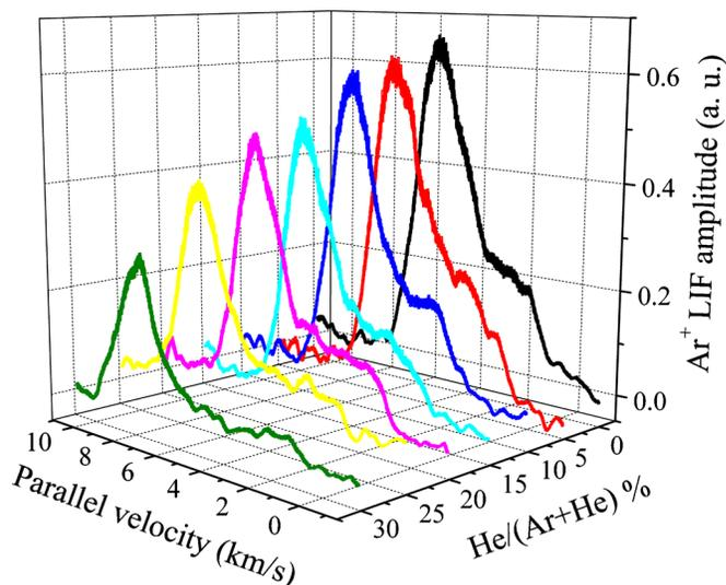
FIG. 8. (Color online) Effect of increasing helium fraction on the Ar<sup>+</sup> parallel ivdf in HELIX. Measurements were obtained at  $z=146$  cm.
