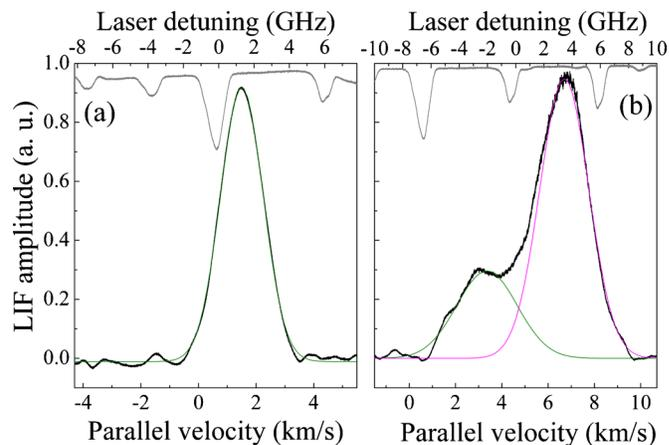
FIG. 2. (Color online) Argon ion parallel velocity distribution functions in (a) HELIX at  $z=126\text{ cm}$  and (b) HELIX at  $z=146\text{ cm}$ . The thick black lines are LIF signals; the thin lines are Gaussian fits assuming a single and a dual ion population line; and at the top is the iodine reference spectrum. The ivdf evolves from unimodal at  $z=126\text{ cm}$  into bimodal at  $z=146\text{ cm}$ .
