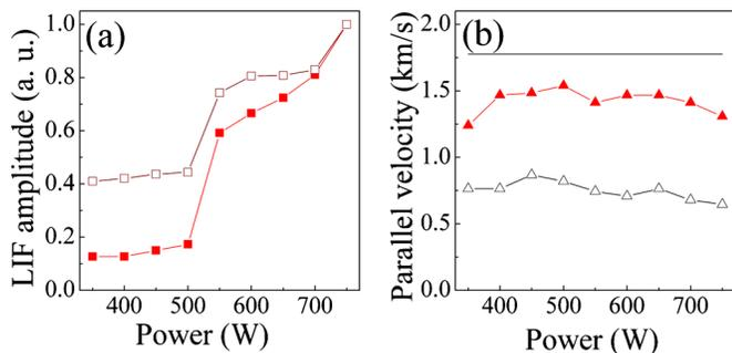
FIG. 7. (Color online) (a) Normalized Xe<sup>+</sup> LIF signal amplitude and (b) Xe<sup>+</sup> parallel flow speed vs input rf power in HELIX at  $z=126$  cm (open symbols) and  $z=146$  cm (filled symbols). (b) Xe<sup>+</sup> Bohm speed at  $z=126$  cm. Operating conditions:  $f=9.5$  MHz,  $B_H=700$  G,  $B_L=10$  G, and  $p_H=1.3$  mTorr.
