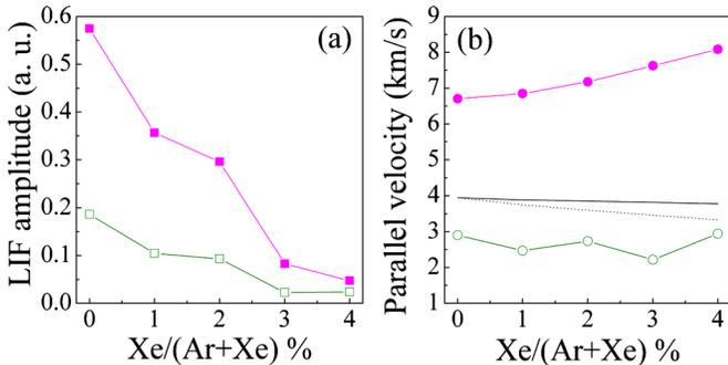
FIG. 4. (Color online) At  $z=146$  cm in HELIX, the Ar<sup>+</sup> LIF amplitude (a) and parallel flow speed (b) as function of small changes in the xenon fraction. Filled and open symbols denote the fast and slow ion group, respectively. (b) The Ar<sup>+</sup> (solid line) and system (dotted line) sound speeds calculated based on measurements at  $z=126$  cm.
