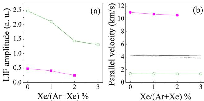
FIG. 5. (Color online) (a)  $\text{Ar}^+$  LIF amplitude and (b) parallel flow speed as function of xenon fraction at  $z=169$  cm in LEIA. Filled and open symbols denote the fast and slow ion groups, respectively. (b) The  $\text{Ar}^+$  (solid line) and system (dotted line) sound speeds calculated based on measurements at  $z=169$  cm.
