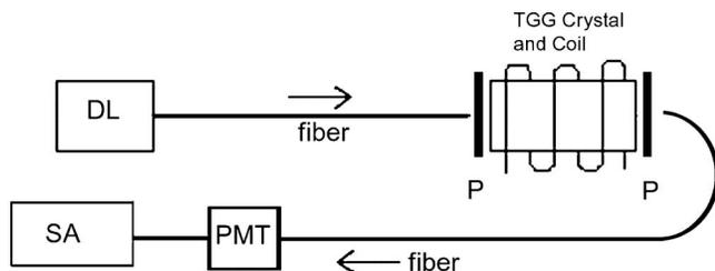
FIG. 3. Dye laser light at 611 nm is coupled into a 200  $\mu\text{m}$  core optical fiber, polarized, and passed through the TGG crystal. Upon exiting the crystal, the light passes through another 1/4 in. diameter polarizer oriented at  $45^\circ$  relative to the first and is coupled into a second fiber that conveys the light to a 10 MHz bandwidth PMT detector whose output is monitored with the spectrum analyzer. (DL: dye laser; P: polarizer; SA: spectrum analyzer).
