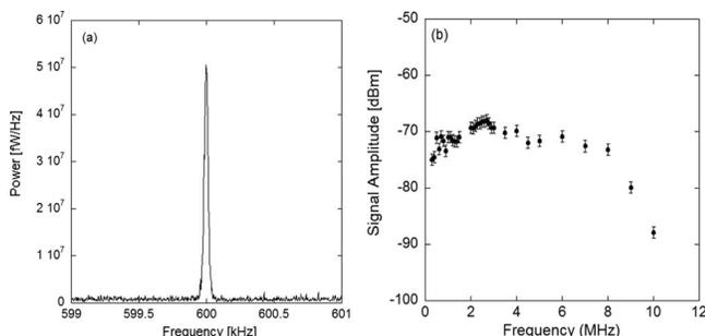
FIG. 4. (a) Typical power spectrum obtained with the fiber coupled, “probe” experimental configuration for a 10 G, 600 kHz modulated magnetic field. (b) Measured signal for a magnetic fluctuation amplitude of 40 G vs modulation frequency.
