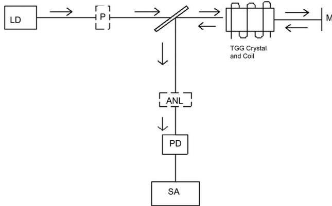
FIG. 1. Schematic of materials testing apparatus. (LD: diode laser; P: polarizer; M: mirror; ANL: analyzer; PD: photodiode; SA: spectrum analyzer).
