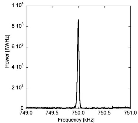
FIG. 2. Power spectrum of the photodiode signal for a 10 G, 750 kHz applied magnetic field fluctuation.
