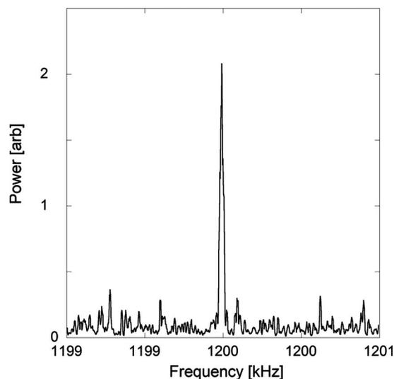
FIG. 5. Power spectrum obtained with the fiber coupled, probe experimental configuration for a 2 G, 1200 kHz modulated magnetic field.
