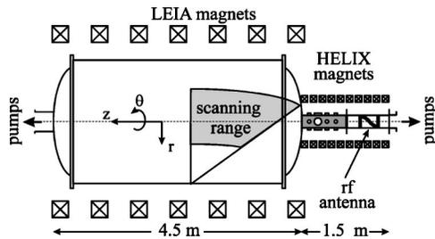
FIG. 1. The combined HELIX-LEIA system with the region accessible with the scanning probe shaded in gray.
