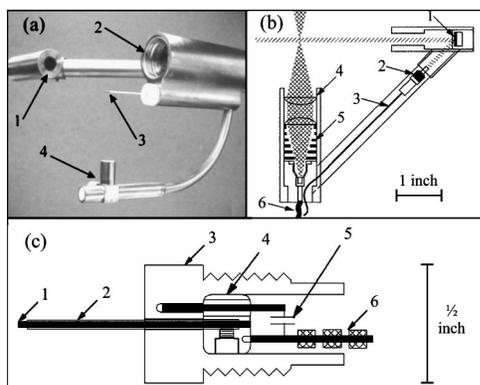
FIG. 2. Scanning probe head diagnostics: (a) 1—LIF injection optics; 2—LIF collection optics; 3—rf compensated Langmuir probe; 4—3D magnetic sense coil array. (b) 1— injection mirror; 2—collimating injection optic; 3— injection fiber; 4—collection lens; 5—light baffles; 6—collection fiber. (c) 1—0.5 mm graphite rod; 2—alumina tube; 3—boron nitride cap; 4—brass slug; 5—10 nF shorting capacitor; 6—rf choke chain.
