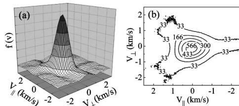
FIG. 3. Tomographic reconstruction of the 2D ion velocity distribution function as surface plot (a) and as contours of constant  $f_i(v_{\parallel}, v_{\perp})$  (b).
