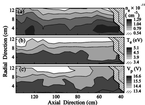
FIG. 4. Two-dimensional maps of plasma density (a), electron temperature (b), and plasma potential (c). Hatched regions are inaccessible by the scanning probe; the junction between the HELIX and LEIA chamber is at  $z=0$ .
