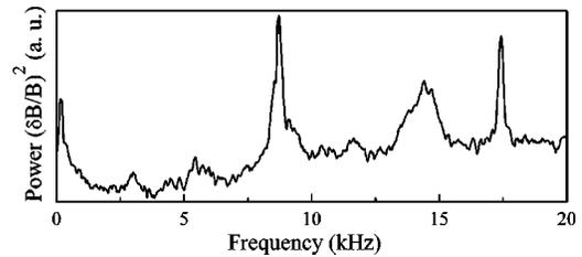
FIG. 5. Magnetic fluctuation power spectrum obtained with one of the three coils in the magnetic sense coil array.
