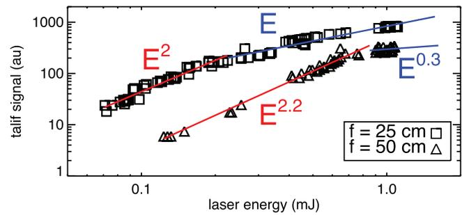
FIG. 1. Measured TALIF signal from KrI (symbols) scales very nearly as  $E^2$  (red curves) until the critical saturation intensity is reached. This occurs for  $E = 0.22 \text{ mJ}$  with an  $f = 25 \text{ cm}$  lens (squares) and  $E = 0.85 \text{ mJ}$  for an  $f = 50 \text{ cm}$  lens (triangles). The critical energy is four times larger in the latter case because the spot size is twice as large.
