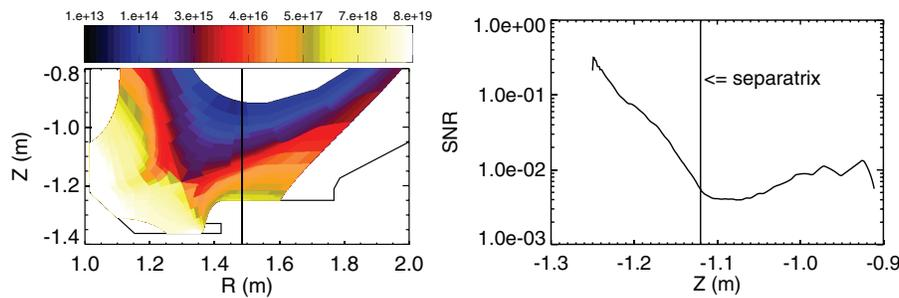
FIG. 3. The neutral density predicted for DIII-D by the UEDGE code in  $\text{m}^{-3}$  (left), and the expected signal-to-noise ratio (right). With averaging, SNR as low as 1% have been resolved in the test plasma, implying that the neutral density can be measured up to the separatrix in DIII-D.
