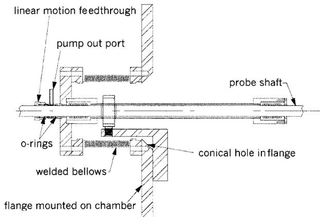
FIG. 2. Mechanical drawing of the entire angular motion feedthrough assembly. The vacuum seal is made on the probe shaft at the linear motion feedthrough with a differentially pumped double O-ring seal. The exterior end of the probe shaft is terminated in a small, sealed chamber with optical and electrical feedthroughs.
