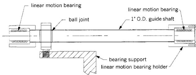
FIG. 1. Mechanical drawing of the ball joint bearing and guide shaft assembly. The principle direction of angular motion is in the plane normal to the drawing.
