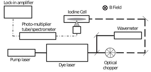
FIG. 2. Optical layout of I-II LIF experiment.
