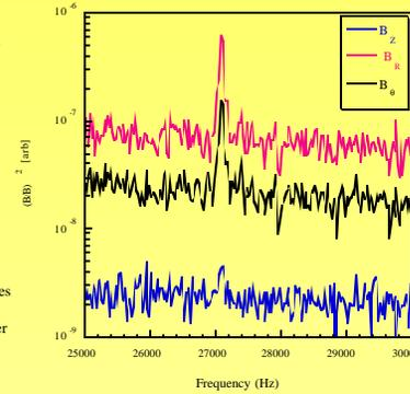
Observed wave polarization consistent with shear Alfvén waves propagating into expansion chamber from source.
