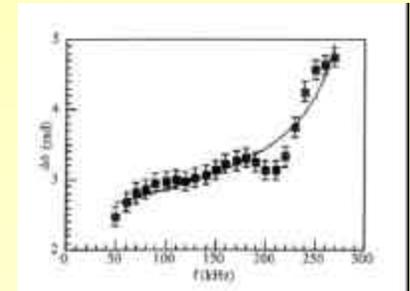
The ion cyclotron resonance in the shear Alfvén wave dispersion has been observed in previous helicon plasma experiments (figure from Watts and Hanna, *Phys Plasmas*, II, 1358 (2004)). In this helium plasma case, the ion cyclotron frequency is 293 kHz and a similar increase in phase difference (wavenumber) is seen near cyclotron resonance.
