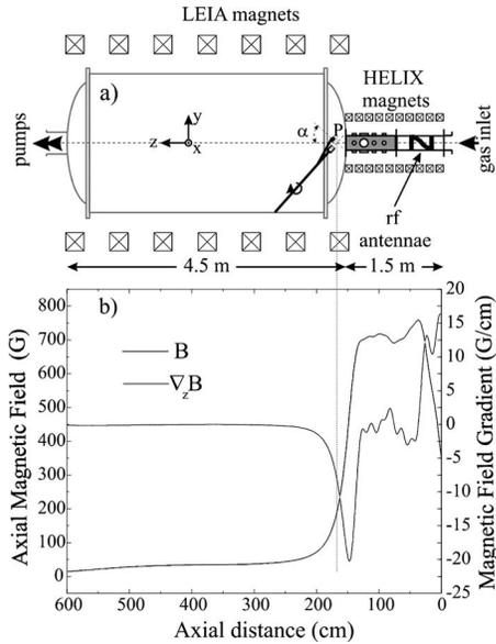
FIG. 1. (a) HELIX diffusion chamber system; (b) the magnetic field profile and the magnetic field gradient on the axis of the system.
