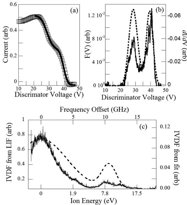
FIG. 3. (a) RFEA data (open squares) and fit of Eq. (4). (b) Derivative of RFEA data with respect to discriminator voltage (solid line) and IVDF obtained from fit of two drifting Maxwellian populations to RFEA data (dashed line). (c) IVDF obtained from fitting of Eq. (4) to RFEA data (dashed line) and LIF measured IVDF (solid line). Lower  $x$  axis is the ion energy after removal of acceleration in the sheath, upper  $x$  axis is the shift in the LIF absorption line.
