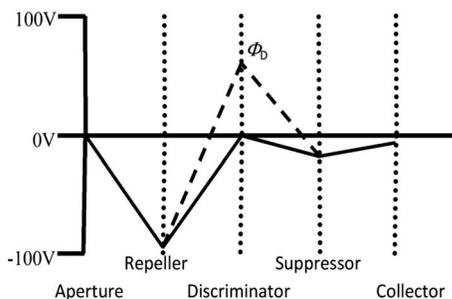
FIG. 2. RFEA bias voltages for each grid (dotted lines). The dashed line indicates the typical range of bias voltages applied to the discriminator.
