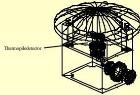
Detector is made of stainless steel with a 1 mm aperture to obtain a spatially resolved beam profile.
