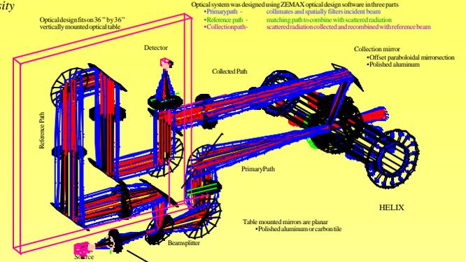
Optical system was designed using ZEMAX optical design software in three parts
