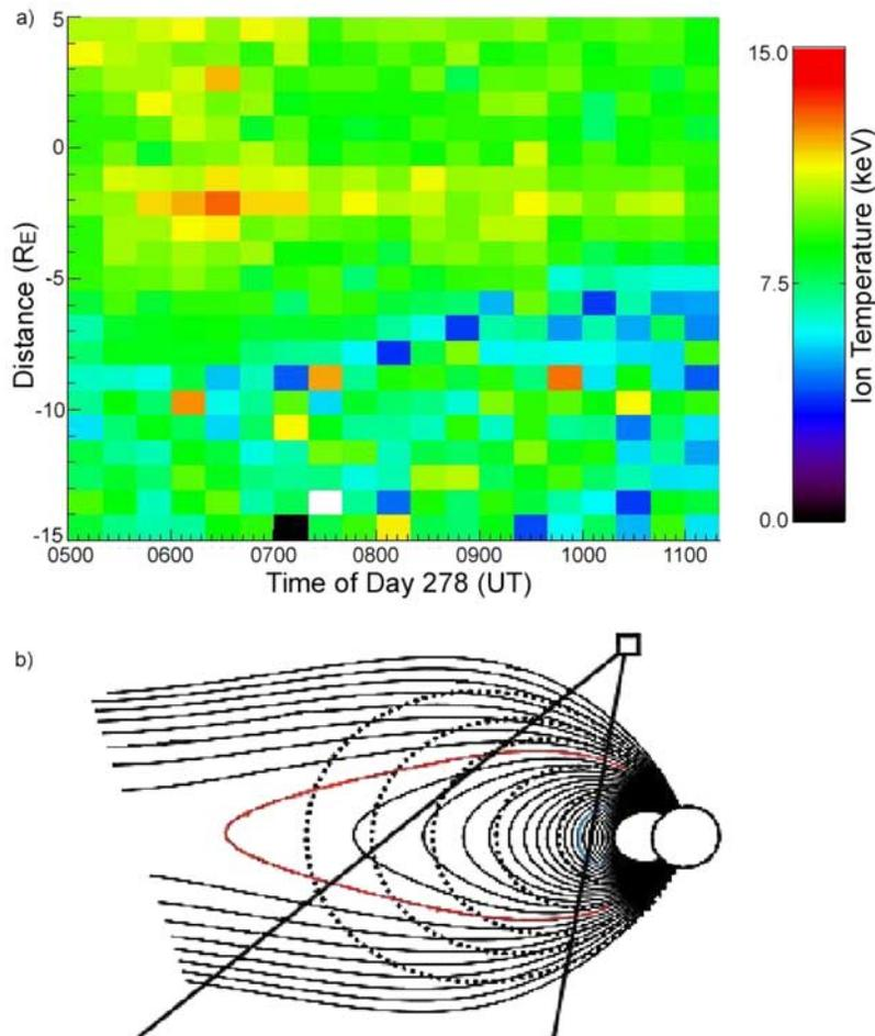
**Figure 5.** (a) Similar to Figure 3a, except the pixels along the  $x$  axis are 20 min averages of MENA data, and they are combined into  $1 R_E$  bins along the  $y$  axis. (b) MENA lines of sight in relation to the magnetic field. Dipole field lines (dashed) for  $L = 4, 6, 8, 10,$  and  $12$  and field lines from the Tsyganenko-96 model (solid) are shown (adapted from *Brandt et al.* [2002]).
