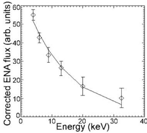
**Figure 1.** Energetic neutral atom (ENA) flux corrected by the energy dependent charge-exchange cross sections versus energy bin (diamonds) and the corresponding Maxwellian fit used to obtain the ion temperature.
