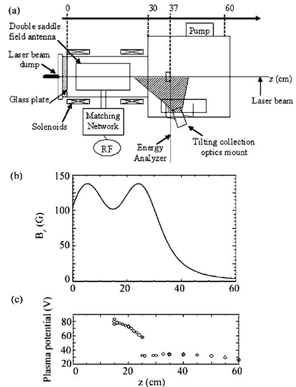
FIG. 2. (a) Chi-Kung apparatus with field of view of LIF collection optics shown as the shaded region. (b) Magnetic field geometry shown for strong magnetic field ( $I_B=6$  A in both coils) case. (c) Plasma potential versus axial position in Chi-Kung showing double layer potential drop for  $P=0.2$  mTorr,  $P=250$  W, and strong magnetic field case (Ref. 1).
