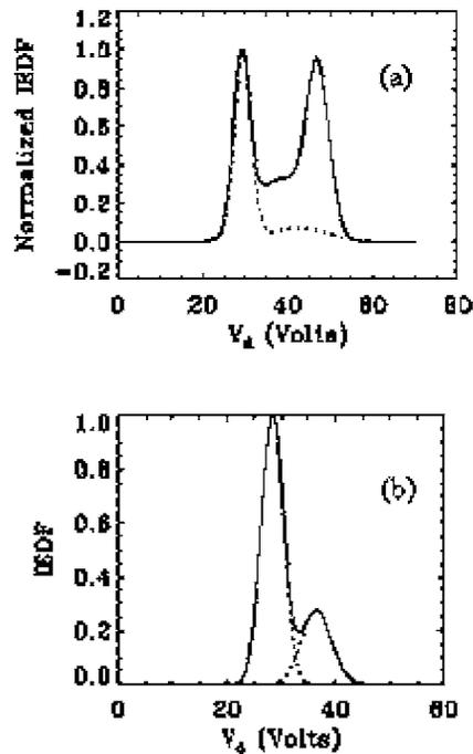
FIG. 1. Normalized IEDFs obtained with the RFEA at  $P=250$  W and the strong magnetic field case. (a)  $z=37$  cm (solid line) and  $z=50$  cm (dashed line) for  $P=0.35$  mTorr. (Ref. 3). (b)  $z=37$  cm for  $P=1$  mTorr. The dashed line is a Gaussian fit to each peak.
