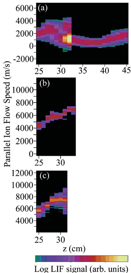
FIG. 5. (Color) Logarithm of LIF signal versus parallel argon ion flow speed (away from the source) and axial position for (a)  $P=1.3 \text{ mTorr}$ , weak magnetic field case, (b)  $P=0.55 \text{ mTorr}$ , strong magnetic field case, and (c)  $P=0.37 \text{ mTorr}$ , strong magnetic field case. rf power is 740 W in all cases.
