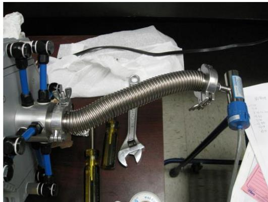
Figure 7: Convectron gauge attached to pump inlet.
