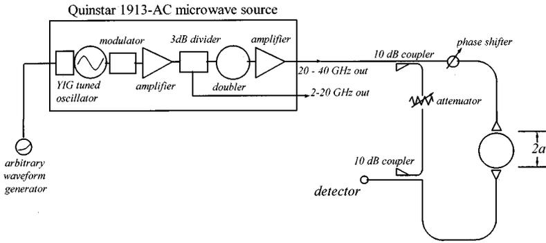
FIG. 1. Schematic of the microwave system including the source and waveguide structures.
