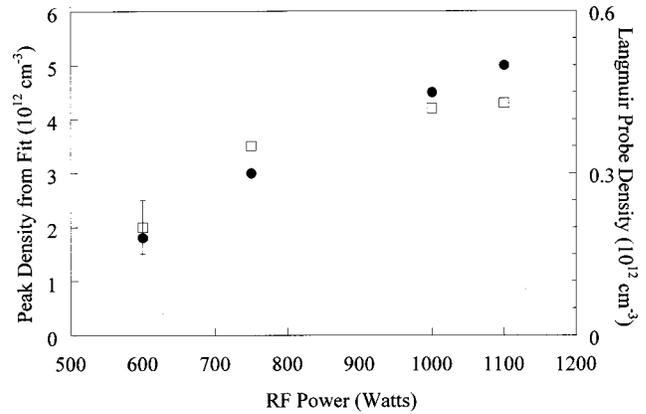
FIG. 8. Comparison of the peak density obtained from the swept frequency microwave system (open squares) and the downstream density measured with a Langmuir probe (filled circles) as a function of source rf power. A typical error bar representative of the uncertainty in the numerical fit is shown for the data point at 600 W. The statistical errors in the Langmuir probe data are smaller than the size of the data points used.
