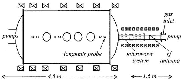
FIG. 3. Schematic of the combined helicon source and space plasma simulation chamber apparatus. The microwave horns are inside the vacuum system at the port indicated. The Langmuir probe measures the downstream plasma density in the space simulation chamber and the laser induced fluorescence system measures the qualitative density profile at the location of the large port adjacent to the microwave system.
