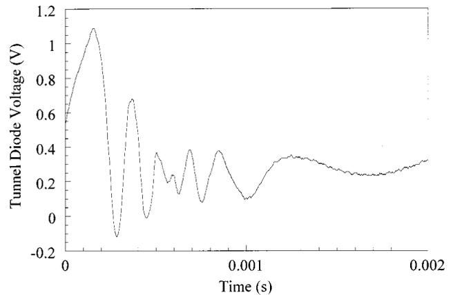
FIG. 4. Tunnel diode signal during pulsed plasma operation showing seven  $2\pi$  phase shifts for 33.6 GHz microwaves.
