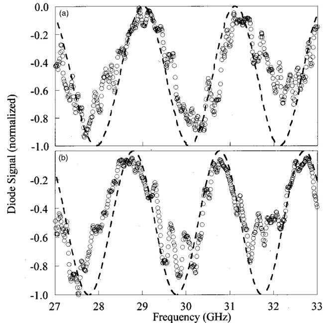
FIG. 6. (a) Beat pattern obtained without plasma. (b) Beat pattern obtained with plasma. Dotted lines are nonlinear fits of Eq. (7) to the measurements.
