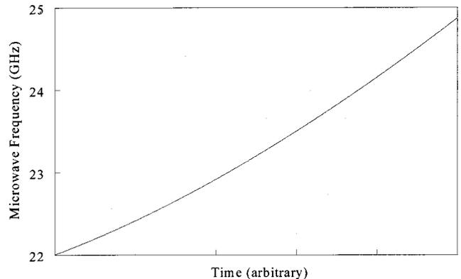
FIG. 2. Typical nonlinear frequency sweep that satisfies the constant beat frequency requirement described by Eq. (5). In this case, a waveguide cutoff frequency of 20.37 GHz was used.
