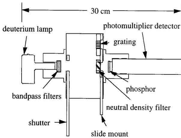
FIG. 1. The compact 121.6 nm light source.
